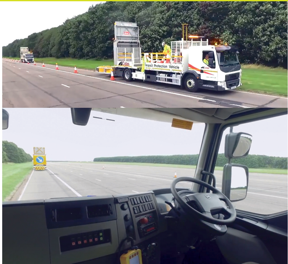
The driverless Colas AIPV travelling as part of a leader-follower pair
